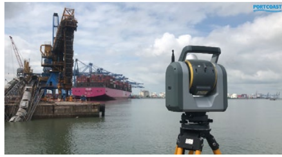
Figure 4 The adoption of Terrestrial Laser Scanning technology in surveying practices; A higher degree of detail and accuracy in surveying
