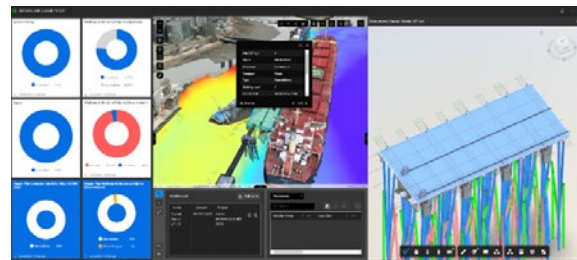
Figure 11 Manage re-construction progress on the ArcGIS platform with integrated BIM (design) model
