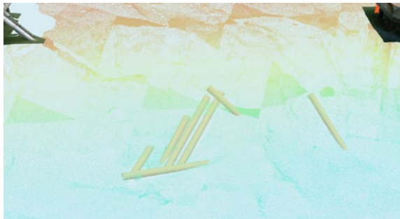
Figure 10 Broken pile segments at sea bed, scanned from USVs devices and integrated into ArcGIS Pro
