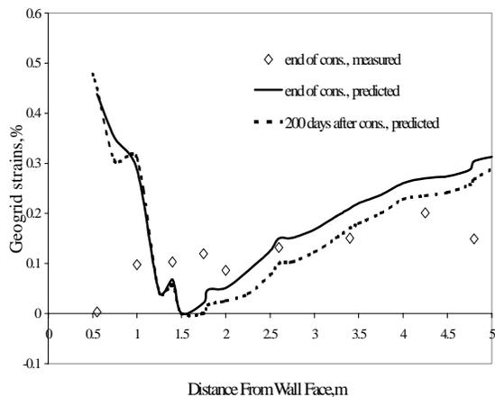
Fig. 8b. Predicted and Measured Strains of Mat 2
