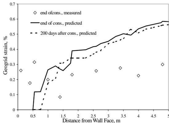
Fig. 8a. Predicted and Measured Strains of Mat 1
