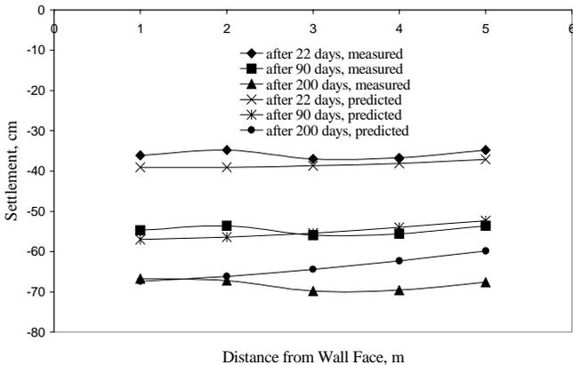
Fig. 4. Predicted and Measured Surface Settlements versus Time and Location
