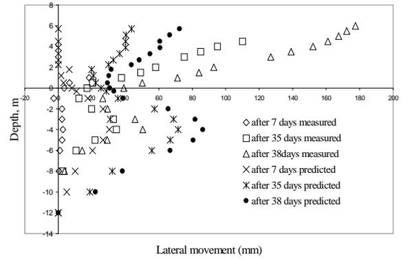
Fig. 5. Predicted and Measured Lateral Movements at Face versus Time During Construction
