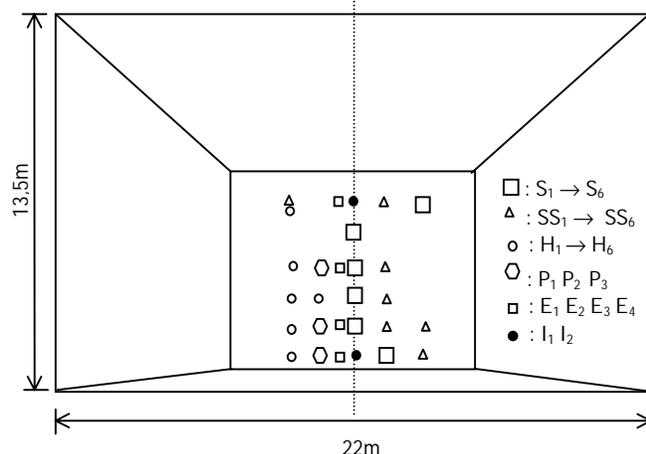
Fig. 1. Instrumentation Layout Plan of Geogrid Test Embankment
