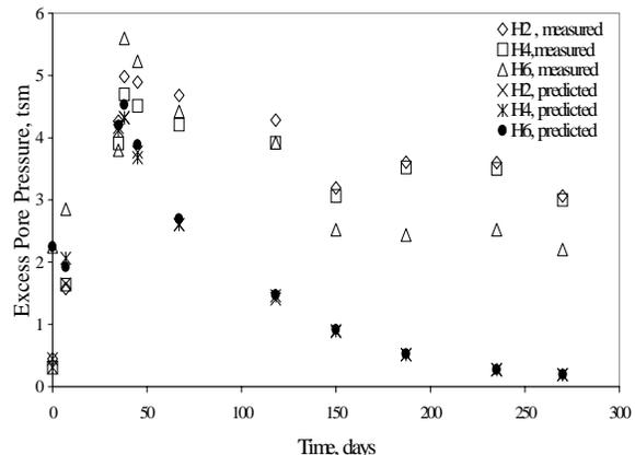
Fig. 7. Variation of Excess Pore Pressure at 6m depth Measurement and Prediction
