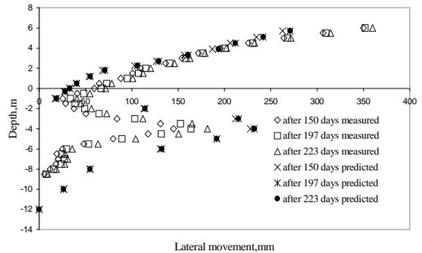
Fig. 6. Lateral Movement at Face After Construction and at Different Time After Construction
