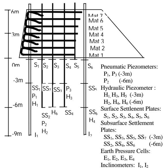
Fig. 2. Schematic Diagram of The Instrumented Geogrid Test Wall Embankment.
